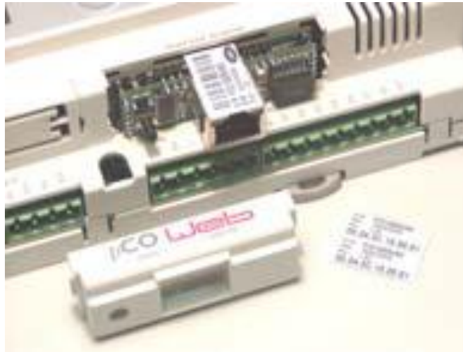
Figure 1.c – Inserting pCOWeb in the pCO controller
