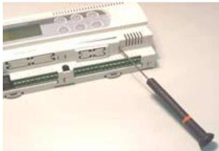
Figure 1.b – Removing the cover from the pCO controller
