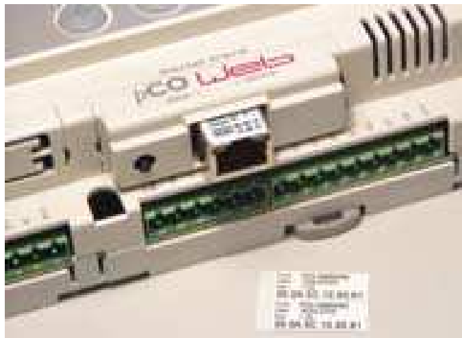
Figure 1.d – Securing pCOWeb with the cover
