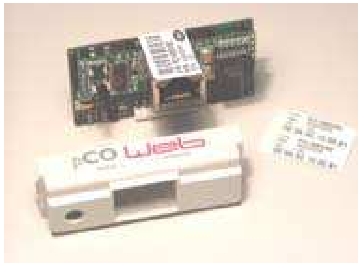
Figure 1.a – pCOWeb and the accessories supplied
