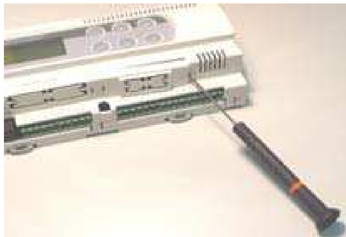
Figure 1.b – Removing the cover from the pCO controller
