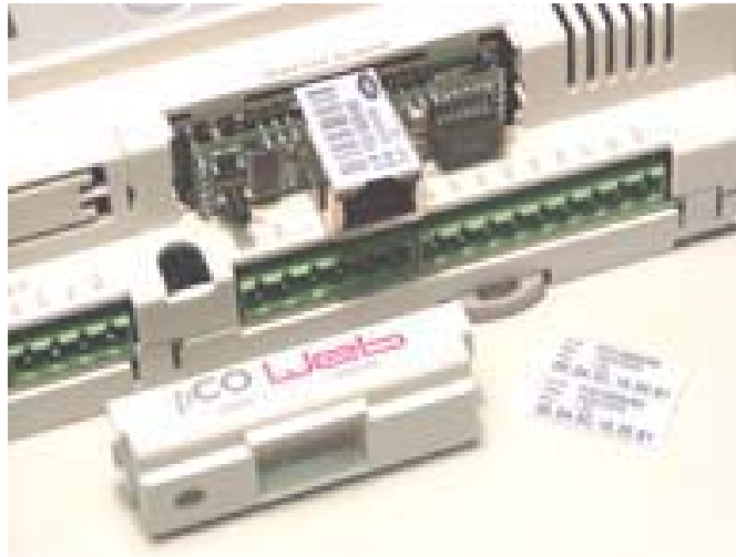
Figure 1.c – Inserting pCOWeb in the the serial cart slot of the pCO controller
