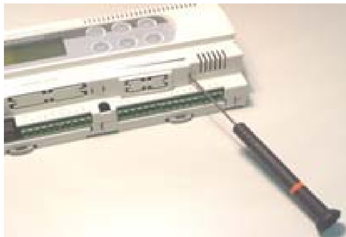
Figure 1.b – Removing the cover from the pCO controller
