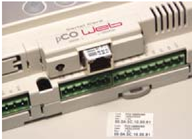
Figure 1.d – Securing pCOWeb with the cover
