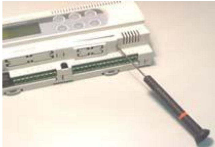
Figure 1.b – Removing the cover from the pCO controller
